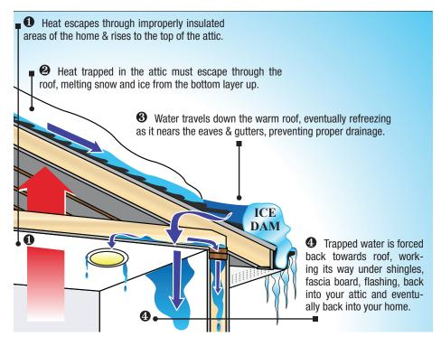
During Winter, attics should act as a buffer zone between the warm interior of your home and the very cold outside temperatures. The temperature inside your attic during this time of year should stay as close as possible to the temperature outside, or as close as possible to 32°F. As the temperature inside your attic goes up, the chances of ice daming increase.
